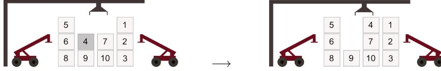
**Fig. 2.** Left: The classically pre-marshalled container bay from Fig. 1, now serviced by reach stackers. The shaded container is blocked horizontally. Right: A configuration where all containers can directly be removed by reach stackers.
